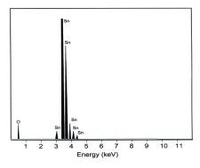
Fig. 1 - EDS analysis of SnO<sub>2</sub> calcined at 400 °C
